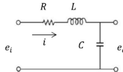
素子方程式  $v_R = Ri, \quad v_L = L \frac{di}{dt}, \quad v_C = e_o = \frac{1}{C} \int_0^t i(t) dt$
